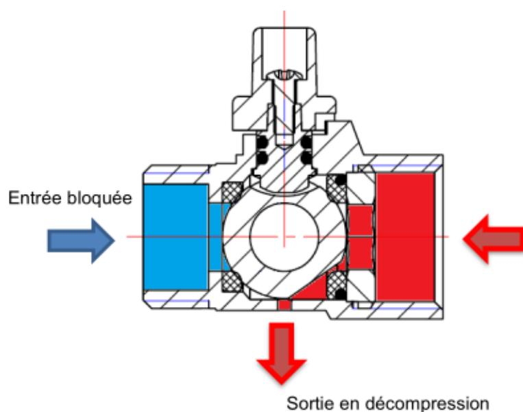
**MINI VANNE A SPHERE LAITON 4MS A DECOMPRESSION MALE FEMELLE BSP**
