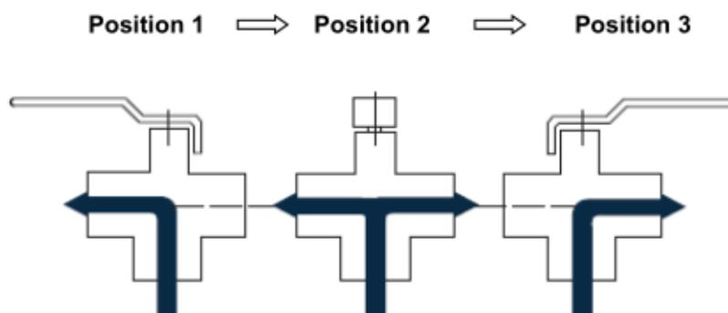
**VANNE A SPHERE 3 VOIES EN T LAITON 4MS 3 POSITIONS PN25 TARAUEE BSP**
