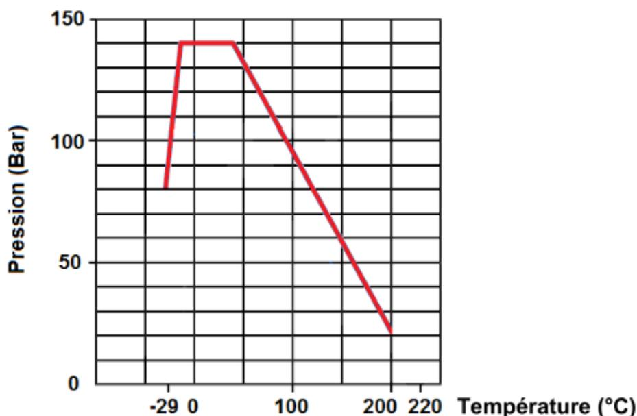
**ROBINET TOURNANT SPHERIQUE 3 PIECES ACIER A105N FORGE SWING 800LBS NPT-SW**
