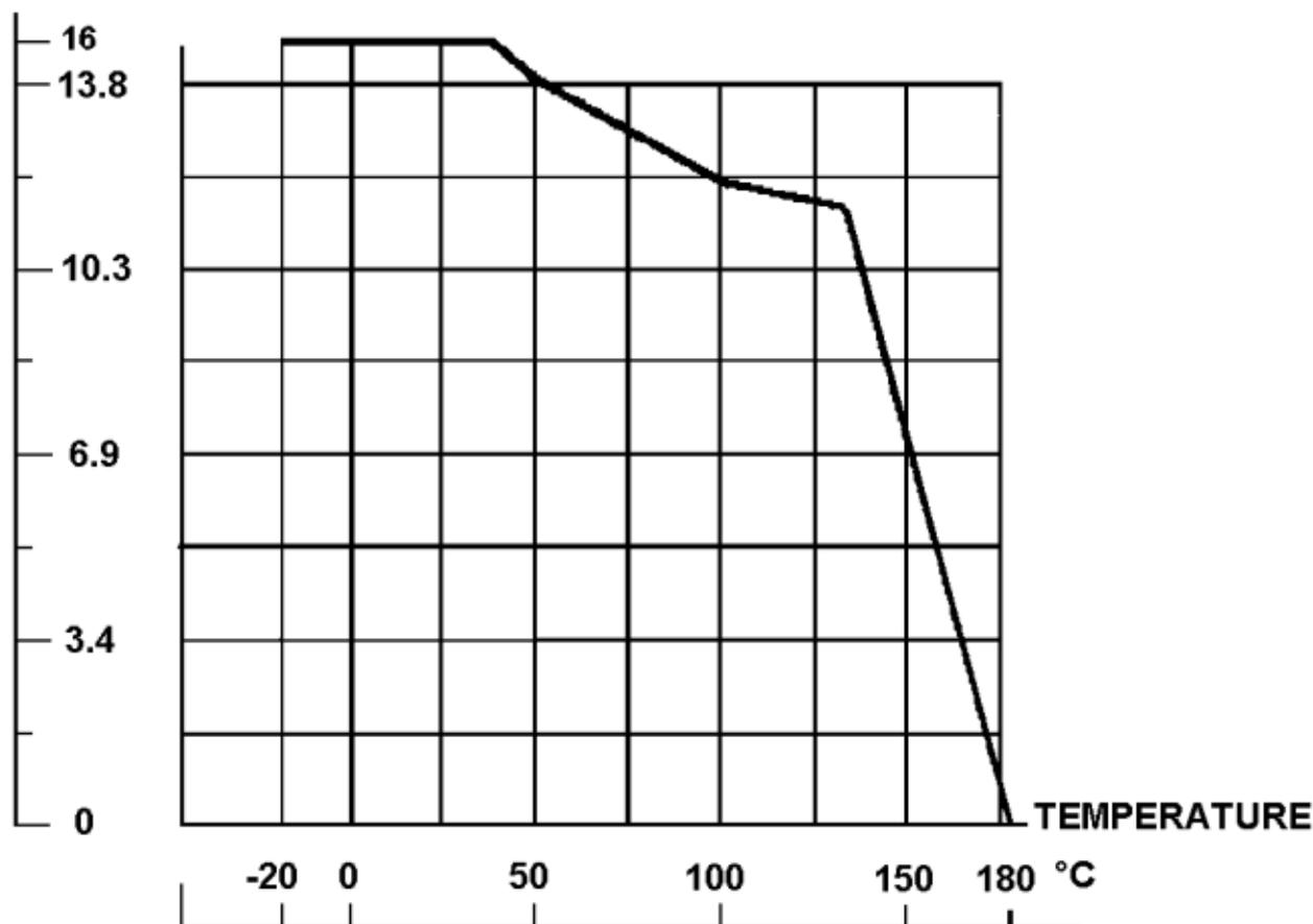
**ROBINET A TOURNANT SPHERIQUE 2 PIECES WAFER MODELE ETROIT INOX PN16**
